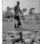
PHOTO COURTESY / MUSTAFA DAFALLA AND ZAHIR DOSSA A Sudanese farmer operates a treadle-powered foot pump.
