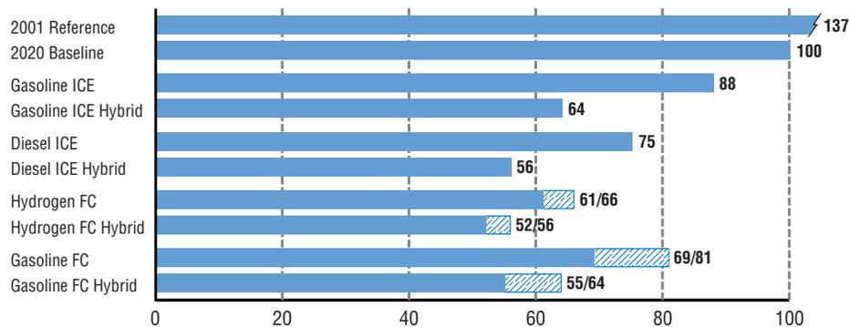
in capacity and performance to a Toyota Camry in 2020, assuming “evolutionary” changes in the engine, vehicle body, and fuel. All the other vehicles assume more aggressive advances. The hydrogen FC technologies assume that hydrogen is produced by reforming natural gas at local filling stations; it is then compressed for charging vehicle tanks. The gasoline FC technologies assume that gasoline is fed onto the vehicle and converted to hydrogen inside an onboard fuel processor.
